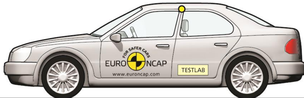
Figure 7-15: Reference point and direction relative to the VUT for dooring scenario
