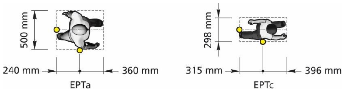
Figure 3-4: Virtual box dimensions around EPTa and EPTc
